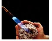
With a flame spread of 25 or less, Greenfiber has a Class 1 Fire rating. Walls with Greenfiber insulation are one-hour (or greater) fire walls and can help control the spread of fire. Greenfiber also has a very low smoke development index level.
