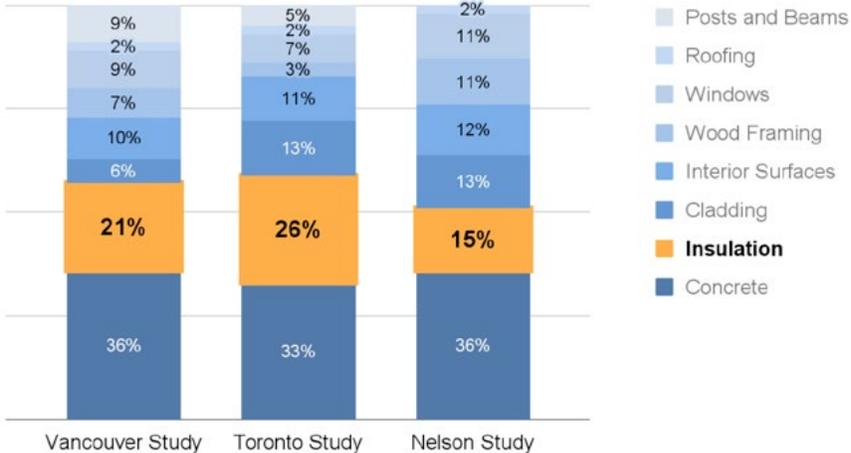
Figure 1 Emissions from home construction based on 550 as-built homes from studies by Builders for Climate Action in 2021-2022
