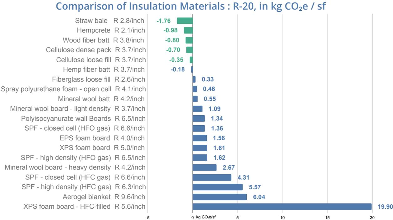
Figure 2 BEAM comparison of insulation materials at R-20, in kg CO<sub>2</sub>e/sf
