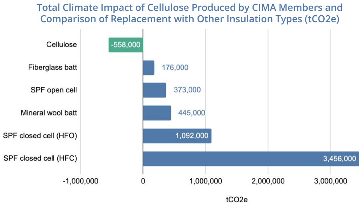
Figure 9 BEAM results for 802 million ft<sup>2</sup> at R-20 thermal performance
